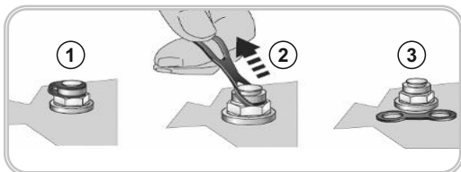
Figure 3: Activation of Vent Plug
