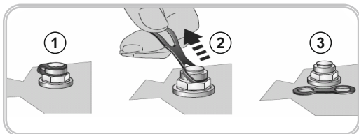
Figure 3: Activation of Vent Plug
