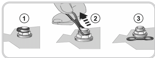
Figure 3: Activation of Vent Plug
