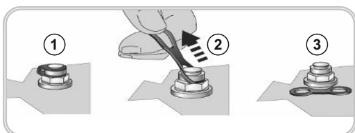
Figure 3: Activation of Vent Plug
