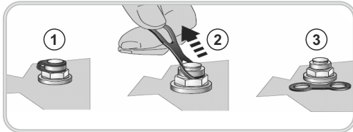
Figure 3: Activation of Vent Plug
